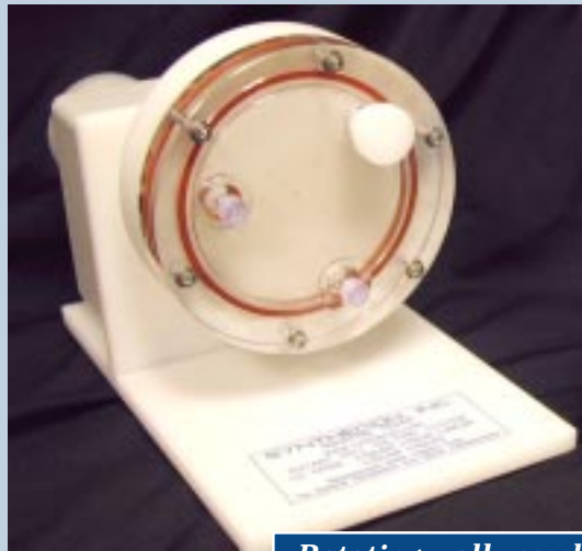
Rotating wall vessel (RWV) bioreactor (Synthecon, Inc., Houston, Texas), which models microgravity.
